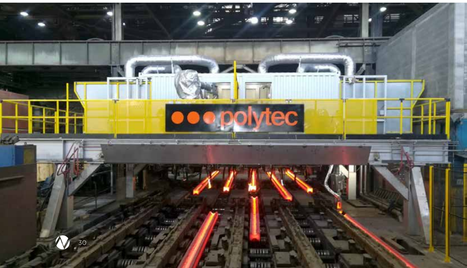
Double billet labelling robot installed at AFV Beltrame Group Vicenza (Italy)
